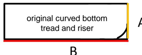
step 3 transfer the measurements onto a riser/s and cut to size iron some matching edging onto the exposed end of riser B (supplied as standard with treads and risers)
