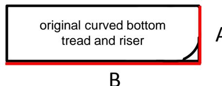
step 2 measure side A (this is the width of your new side riser) measure side B and add 8mm (the front riser will cover the end of the side riser and sit in front of it)
